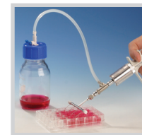
Aspiration with Reverse Modus Valve
